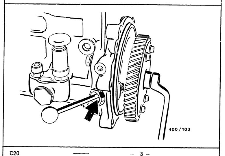
Use extractor KDEP 2918 to detach toothed gear from camshaft. Loosen and unscrew fastening screws of intermediate flange. Remove intermediate flange.
